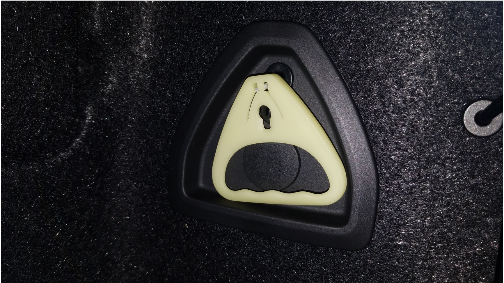
FIGURE 5.8 VEHICLE TRUNK COMPARTMENT MANUAL RELEASE MECHANISM
